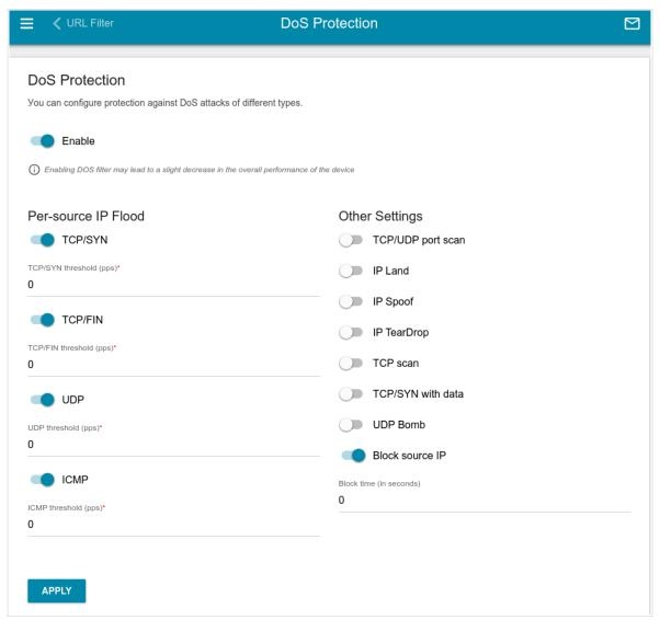
Figure 164. The Firewall / DoS Protection page.
