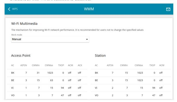
Figure 105. The page for configuring the WMM function.
