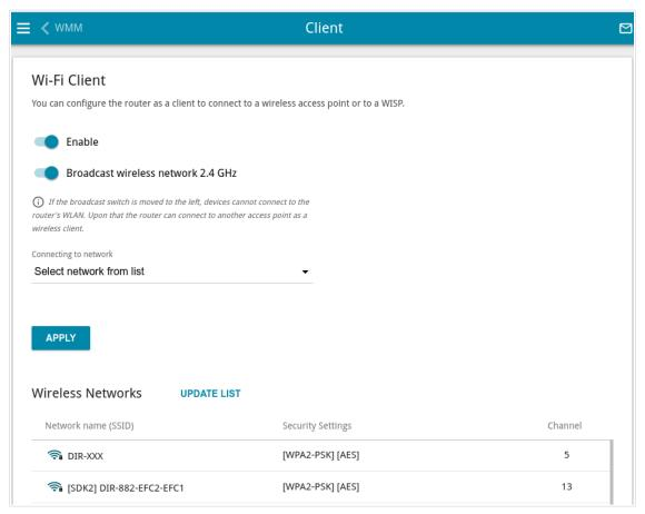
Figure 107. The page for configuring the client mode.
