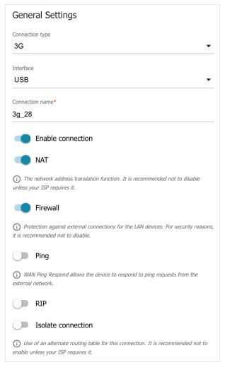
Figure 82. The page for creating a new 3G connection. The General Settings section.
