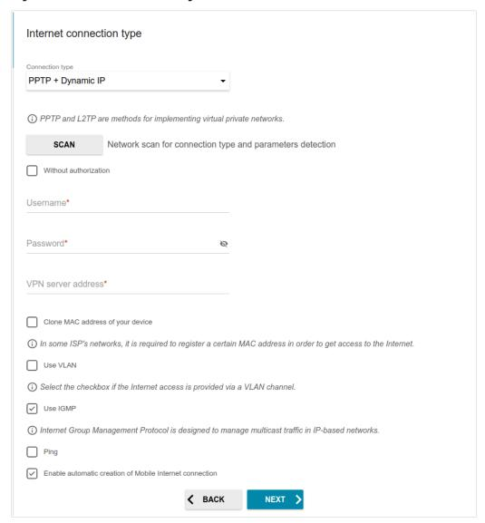
Figure 47. The page for configuring PPTP + Dynamic IP WAN connection.
