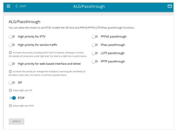
Figure 151. The Advanced / ALG/Passthrough page.
