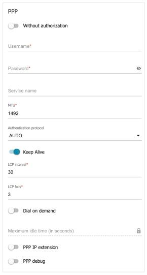
Figure 75. The page for creating a new **PPPoE** connection. The **PPP** section.
