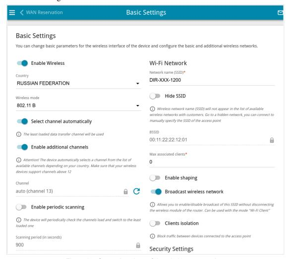
Figure 97. General settings of the wireless connection.
