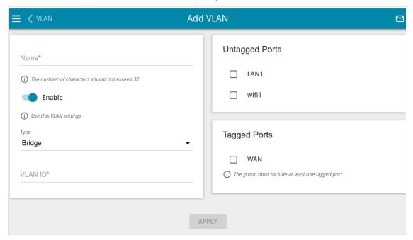
Figure 134. The page for adding a VLAN.
