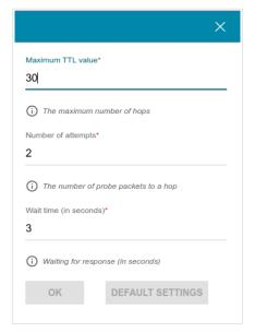
Figure 174. The **System / Traceroute** page. The additional settings window.
