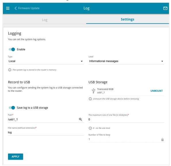
Figure 169. The System / Log page. The Settings tab.
