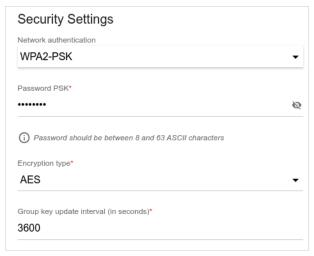
Figure 101. The WPA2-PSK value is selected from the Network authentication drop-down list.
