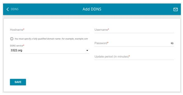
Figure 138. The page for adding a DDNS service.
