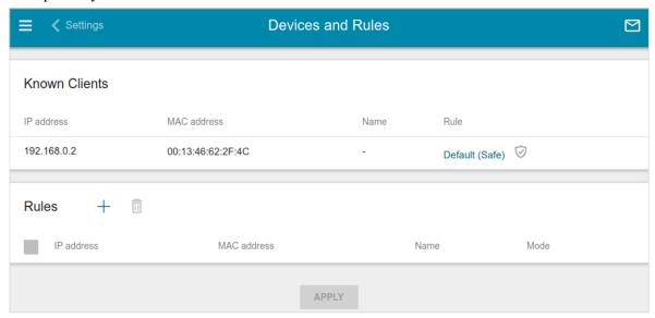
Figure 178. The Yandex.DNS / Devices and Rules page.
