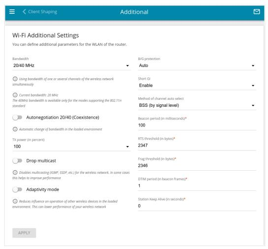
Figure 110. Additional settings of the WLAN.
