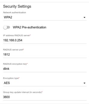
Figure 102. The WPA2 value is selected from the Network authentication drop-down list.
